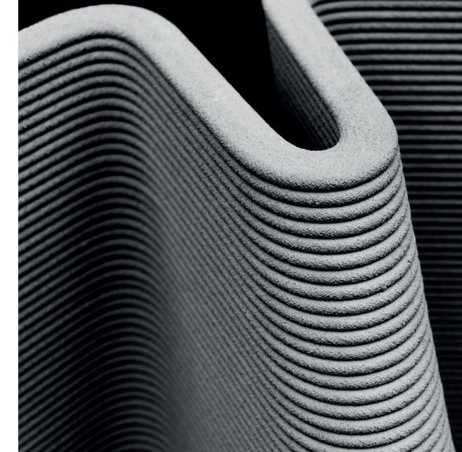
The project aims at developing new solutions for the design and manufacture of urban furniture by 3DP with ecological materials. Design and optimization of shapes will allow a reduction of mortar's quantity. Use of local recycled sand will slow natural resource depletion and avoid landfilling. Substituting natural constituents by recycled ones could reduce the regularity of the printed material and improving online monitoring during printing will allow to compensate the properties variability.
